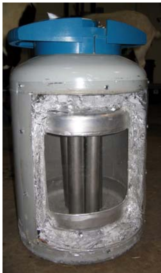
Cutout view of a liquid nitrogen semen storage tank showing insulation and canisters
